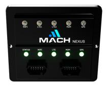
Developed for off-road agricultural, construction and industrial machines, it provides onboard processing and secure connectivity for applications in a wide range of scenarios, such as tractors, ISOBus implements, loaders, skid steers and more. Equipped with a cloud-based management platform, it offers over-the-air (OTA) updates and security, as well as in-field online or offline machine to machine networking and monitoring for autonomous control, logistics, and asset tracking.
