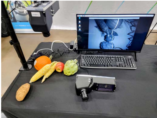
Figure 2: Fruits - Measurement, object identification, detection of damage (bruising)
