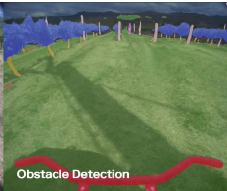
Caption: Prospr's state-of-the-art collision avoidance system integrates LiDAR and cameras to detect and identify obstacles.
